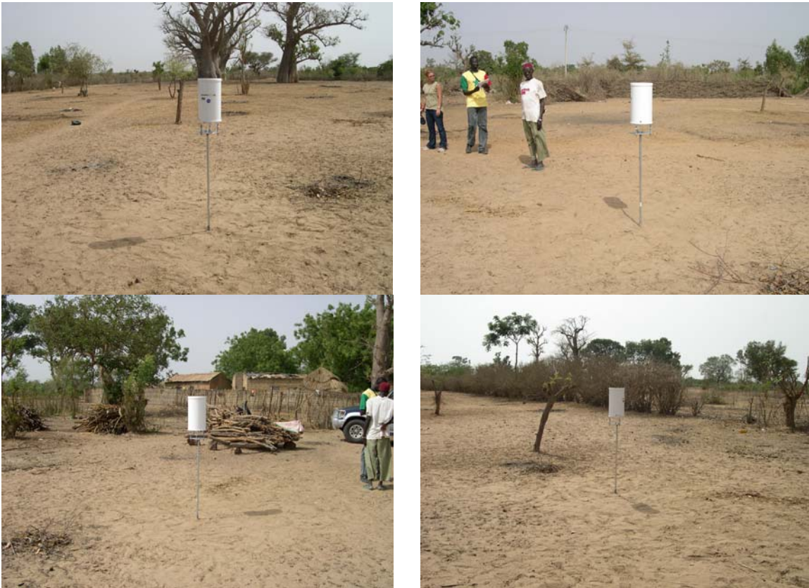
Figure 6: AMMA26 rain gauge site.
