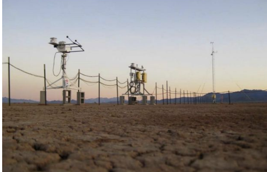
Figure 2: Mobile SURFRAD station at Red Lake, Arizona (Image source: NOAA Global Monitoring Division )
