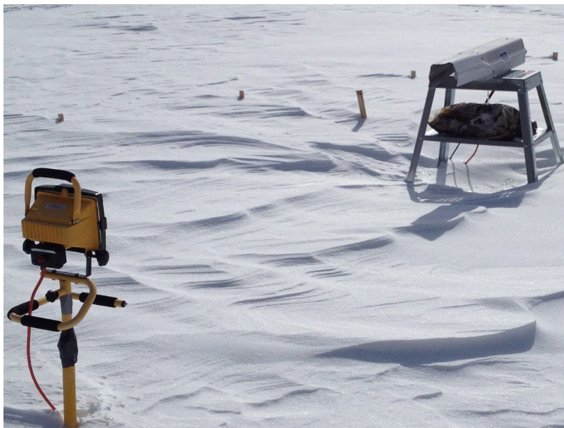
Figure 2: The PIP halogen lamp (left) and high-speed video camera (right) (Image source: GSFC WFF PIP webpage )
