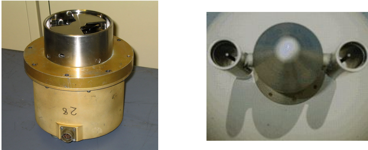
Figure 2. (a) An ER-2 LIP electric field mill & (b) the dual-tube gerdien conductivity probe. (Image sources: Blakeslee, Richard J., Monte Bateman and Douglas M. Mach)
