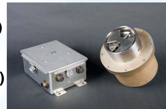
Embedded Linux System (ELS) and Electric Field Mill flown on Global Hawk
