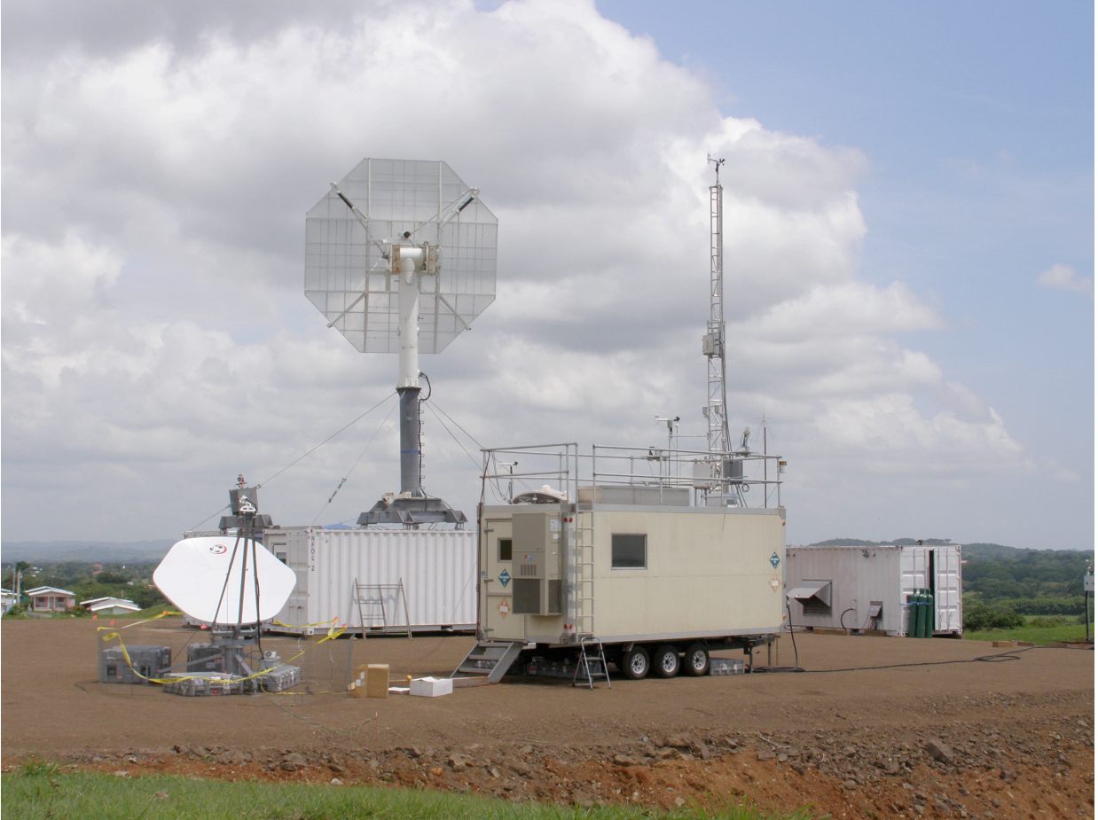
Figure 7. The NASA polarization (NPOL) radar and the NATIVE trailer located in Las Tablas, Panama.
