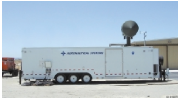
Figure 3.3. —GCS with top-mounted GDT at the El Mirage, CA flight test center.
