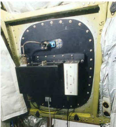
Figure 2. View of the JPL Laser Hygrometer from inside the NASA DC-8 passenger cabin. The box on the right contains the power supplies, and the black box on the left houses the control electronics and instrument computer. A hermetic connector provides the single-cable connection to the optical head. This instrument is autonomous, so an operator is not required to fly on the aircraft.
