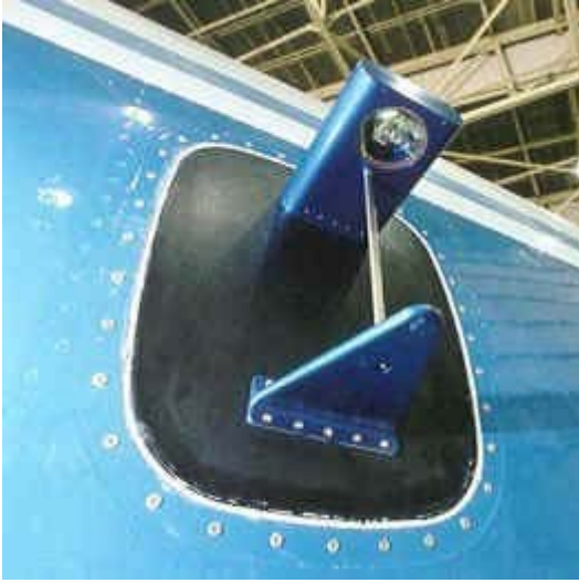
Figure 1. During CAMEX-4, the JLH will be mounted on a DC-8 window port at fuselage station 490 right. To ensure measurements in “clean” air, the optical path is outside the aircraft boundary layer. The laser, detector, and collimating optics are located in the upper housing, with a return mirror on the lower housing. The foreoptics can be evacuated or purged with dry nitrogen to eliminate water vapor absorption inside the optical head. This spectrometer features a simple “there and back” open path between the two external housings, for a total optical pathlength of 50 cm.
