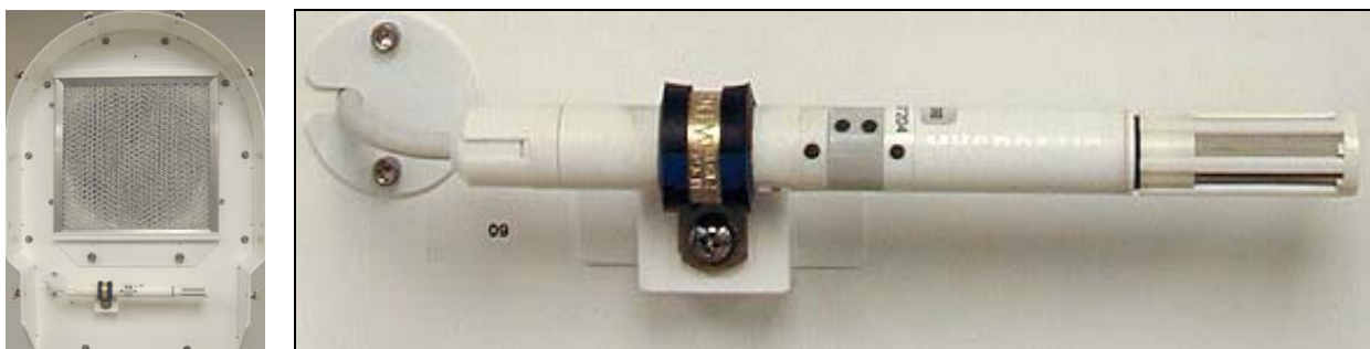
Figure 28. Superblower with End Cover removed; S3 sensor and filter.
