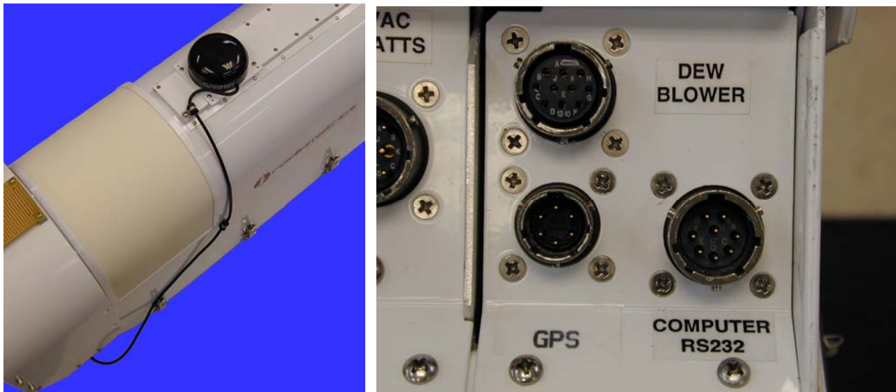
Figure 7. Left: GPS Receiver on WVP-1500. Right: GPS connector on signal panel.
