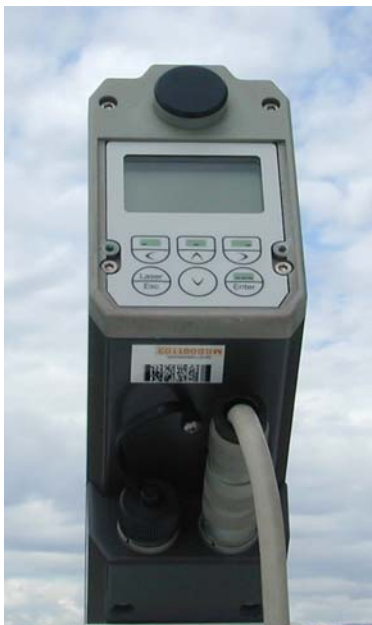
Figure 6. Infrared thermometer and mirror with sun shield removed.
