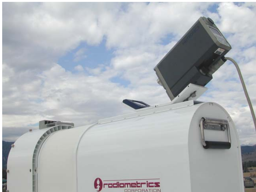
Figure 6. Infrared thermometer and mirror with sun shield removed.
