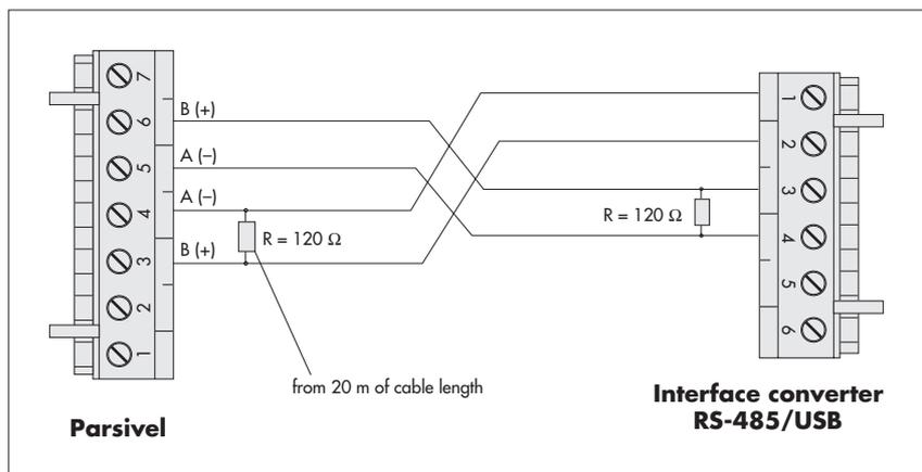
The Parsivel is configured at the factory for 2-wire communication. To switch the Parsivel from 2-wire communication to 4-wire communication, proceed as described in Chapter 8.1 "Connecting the Parsivel to an RS-485/RS-232 Interface Converter (Accessories)".
