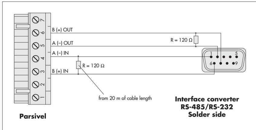
The Parsivel is configured at the factory for 2-wire communication. In order to switch the Parsivel from 2-wire communication to 4-wire communication, proceed as follows:
