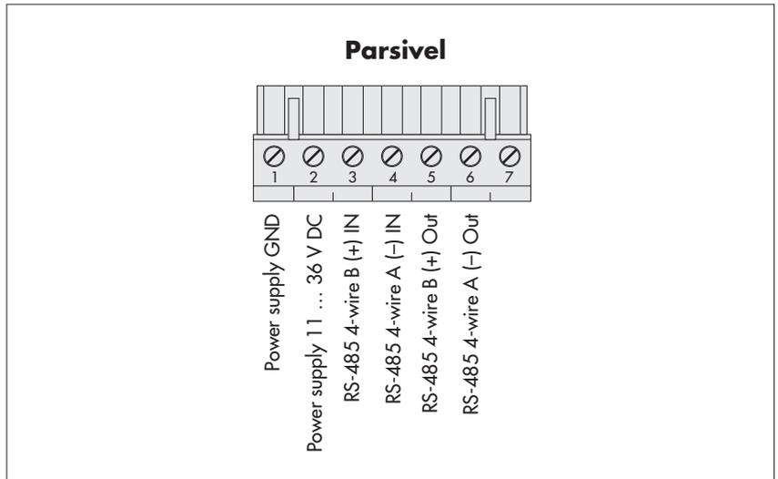
Fig. 4: Connection Assignment for a 2-wire connection with RS-485 of SDI-12 transfer.
