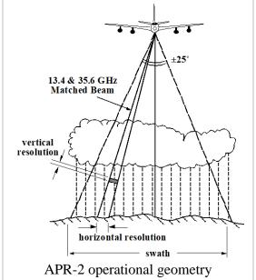
(2003) provides a full description of the APR2 radar system. Calibration of the radar reflectivity products is verified at Ku-band by using the ocean surface and at Ka-band by comparing with the Ku-band reflectivity in light precipitation (Tanelli et al. 2006). Doppler velocities are corrected for aircraft motion using surface return.
