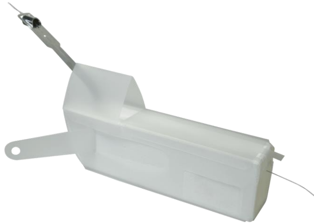
Figure 2: DFM-09 Radiosonde (Image Source: DFM-09 | NORIS Group GmbH )
