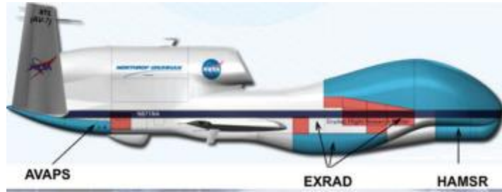
Figure 1: EPOCH airborne instrument suite (Image source: Emory et al., 2015 )
