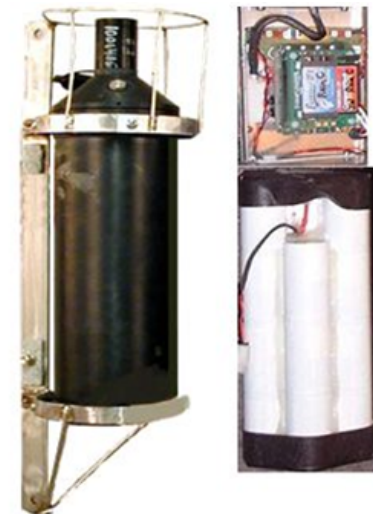
Fig. 1. Passive Aquatic Listener (PAL) deployed over ocean. See Yang et al. (2015) and Riser et al. (2019) for more information about the system configurations.
