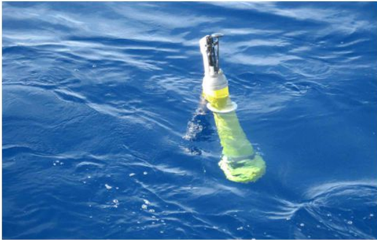
Fig. 1. Passive Aquatic Listener (PAL) deployed over ocean. See Yang et al. (2015) and Riser et al. (2019) for more information about the system configurations.
