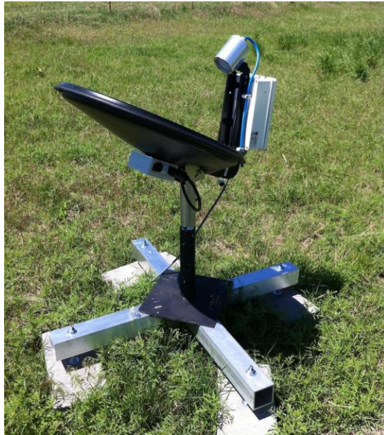
Figure 2: The Micro Rain Radar MRR-2 (Image source: GPM MRR webpage )
