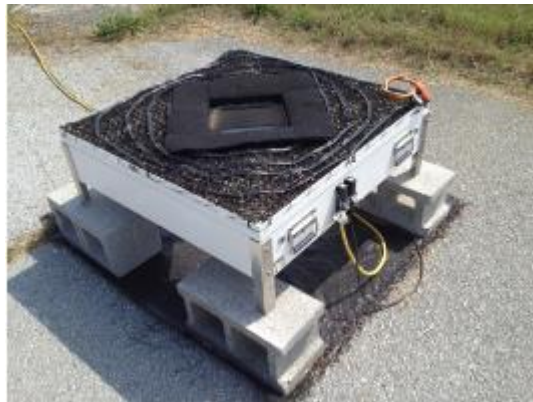
Figure 2: Two-Dimensional Video Disdrometer (2DVD) (Image Source: GSFC GPM webpage )
