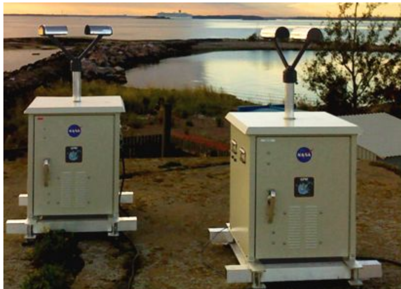
Figure 2: Two Autonomous Parsivel Units (APUs) (Image source: NASA GHRC )
