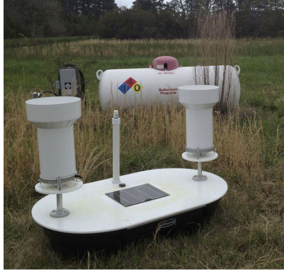
Fig 1: Dual tipping rain gauge bucket used for GPM GV (image source: http://gpm-gv.gsfc.nasa.gov/Gauge/ )
