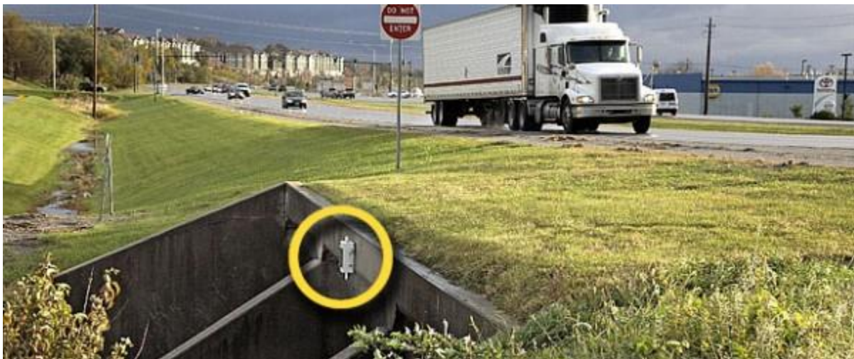
Figure 2: Typical location of the IFC Stream Gauges (Image Source: Iowa Flood Center )
