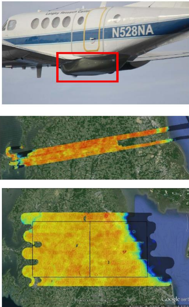
Figure 14 – SLAP aircraft installation and (top panel) and examples of high (200 m) and coarser (1 km) resolution observations for two different flying altitudes.
