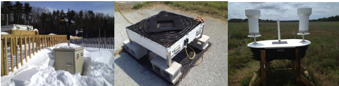
Figure 11 - Pictures of the Automated Parsivel Unit (APU; left), 2DVD (middle) and dual-tipping bucket gauge system (right).
