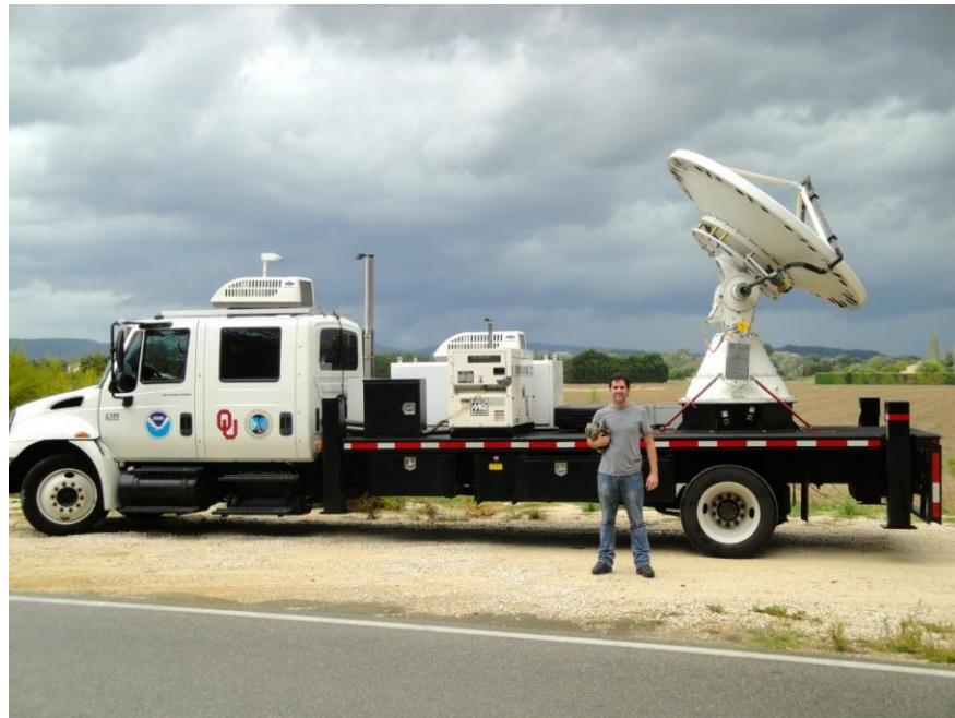
Figure 9 - NOAA NOXP mobile X-band dual-polarimetric radar.
