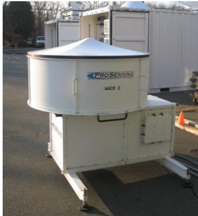
Figure 2: A ProSensing zenith pointing transportable W-band cloud radar (Image source: ProSensing W-band cloud radar webpage )
