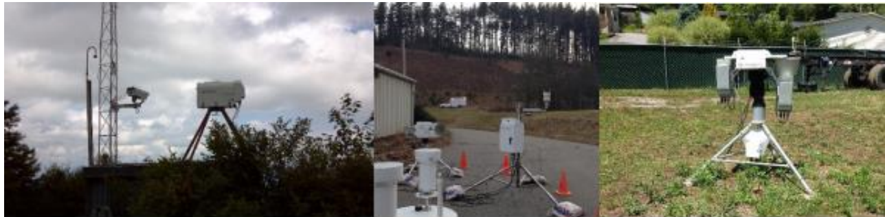
Figure 1: Microwave Radiometer (MWR) instruments. Left to right: MWR 2 channel, eastern MWR 3 channel, and inner region valley MWR 3 channel (Image source: https://www.arm.gov/publications/programdocs/doe-sc-arm-16-008.pdf )
