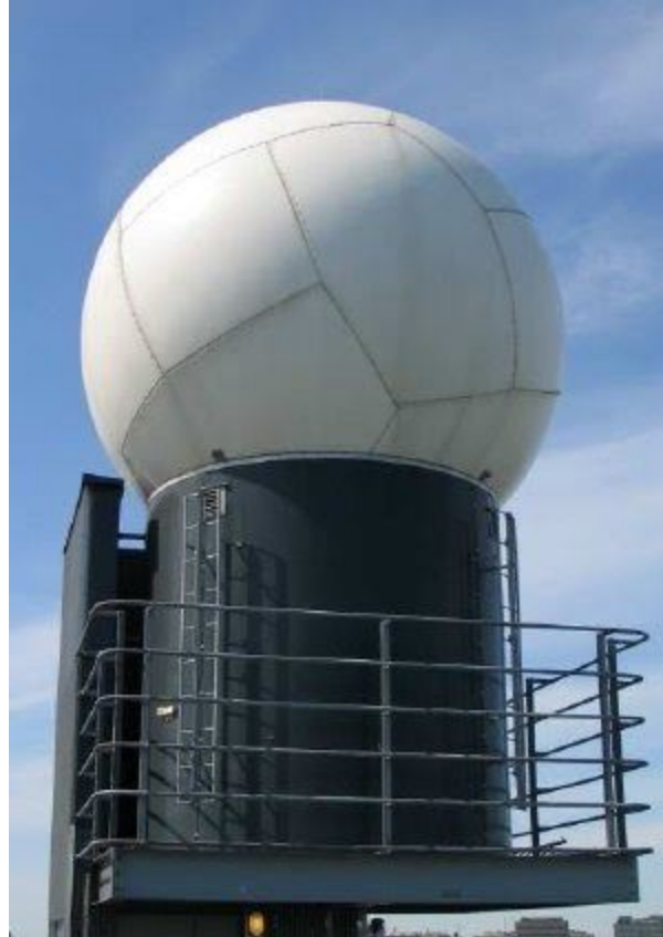
Figure 2: The University of Helsinki Kumpula C-Band Weather Radar (Image source: UH Radar Meteorology Group )
