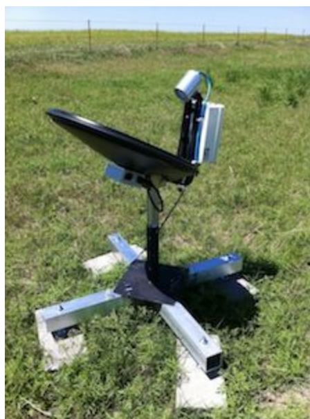
Figure 2: MRR used for GPM Ground Validation (Image source: http://wallops-prf.gsfc.nasa.gov/Radar/MRR/index.html )
