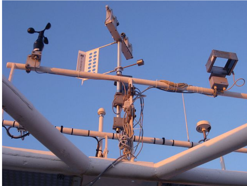
Figure 2: The ODM 470 (top center) along with an anemometer (left) and precipitation detector (right) (Image source: Eigenbrodt ODM 470 webpage )
