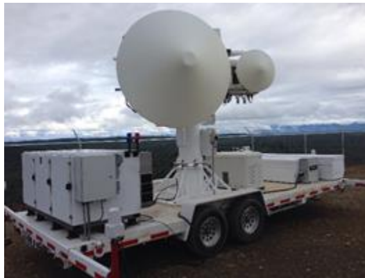
Figure 3: The D3R on its portable trailer during the OLYMPEX field campaign. The smaller (28 inch) antenna is for the Ka-band and the larger (6 ft) antenna is for the Ku-band.
