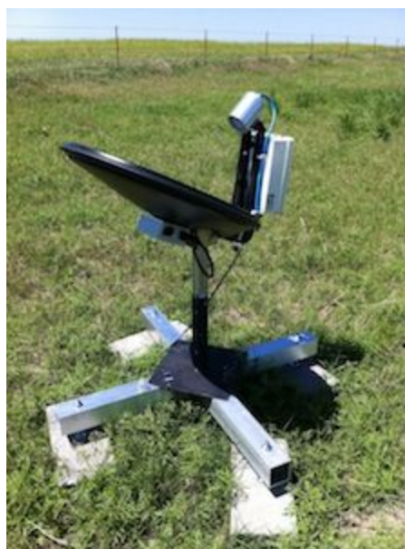
Figure 3: MRR used for GPM Ground Validation (Image source: http://wallops-prf.gsfc.nasa.gov/Radar/MRR/index.html )
