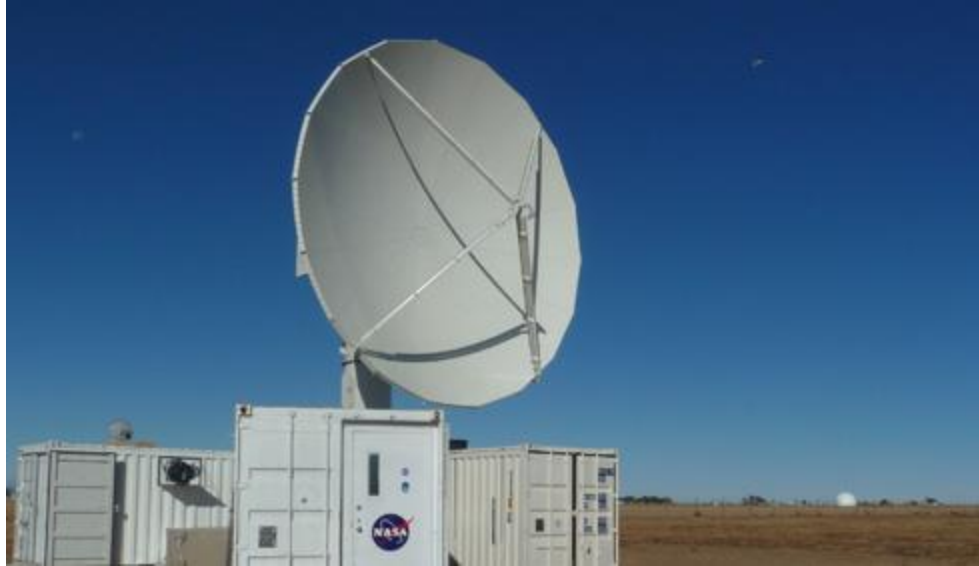
Figure 3: Image of the NPOL Doppler radar (Image Source: Precipitation Measurement Missions NPOL website )
