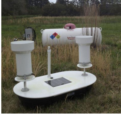
Figure 3: Dual tipping rain gauge bucket used for GPM- GV (Image source: GSFC GPM Rain Gauge webpage )
