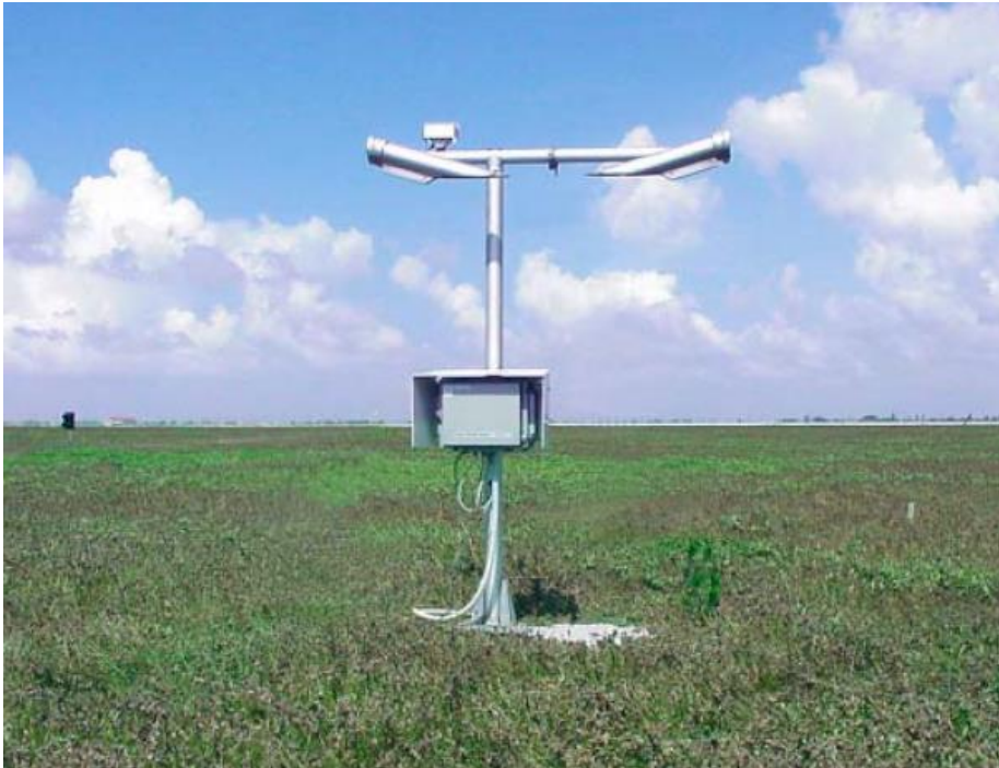
Figure 2: A Vaisala FD12P observation station. (Image source: Vaisala FD12P instrument overview )
