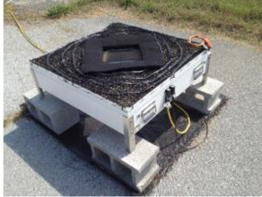
Figure 1: Two-Dimensional Video Disdrometer (2DVD) (Image Source: https://wallops-prf.gsfc.nasa.gov/Disdrometer/index.html )
