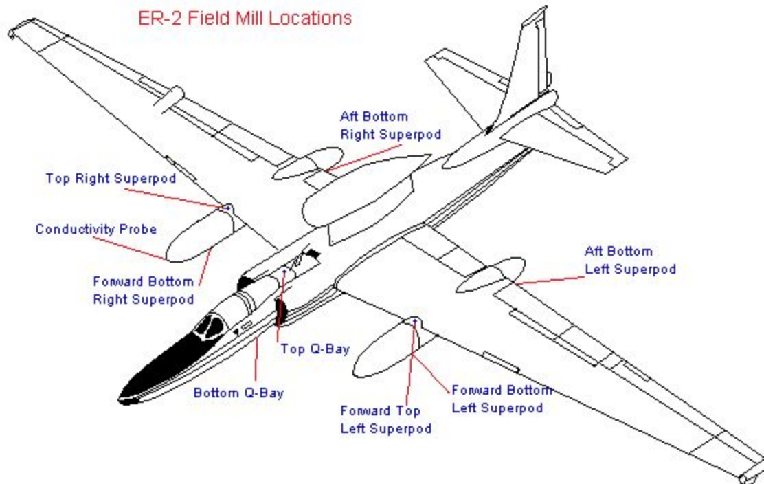
Figure 2: Locations of the eight field mills and the conductivity probe as mounted on the ER-2 aircraft.
