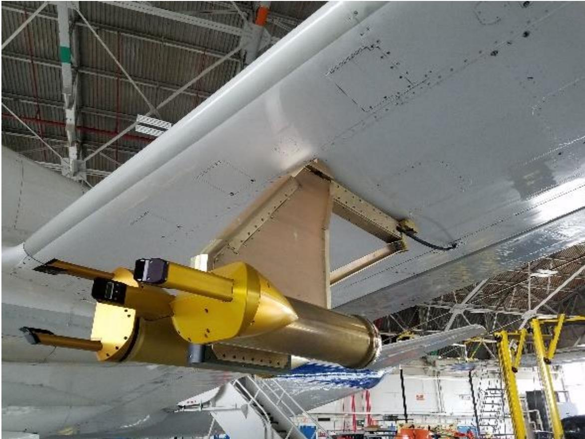
Figure 3: Image of HVPS-3 Instrument
