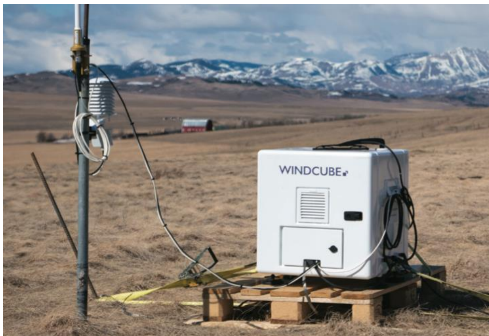
Figure 6: Image of the Leosphere WindCube WLS-10 Series Doppler LiDAR (Image credit: Leosphere )
