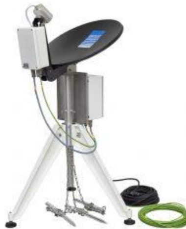
Figure 3: Image of the MRR-PRO instruments (Image source: METEK GmbH Germany MRR-PRO )
