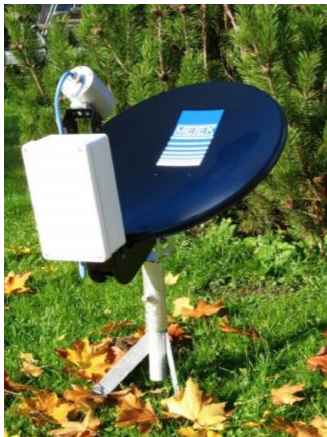
Figure 2: Image of the MRR-2 instrument (Image source: Metek )
