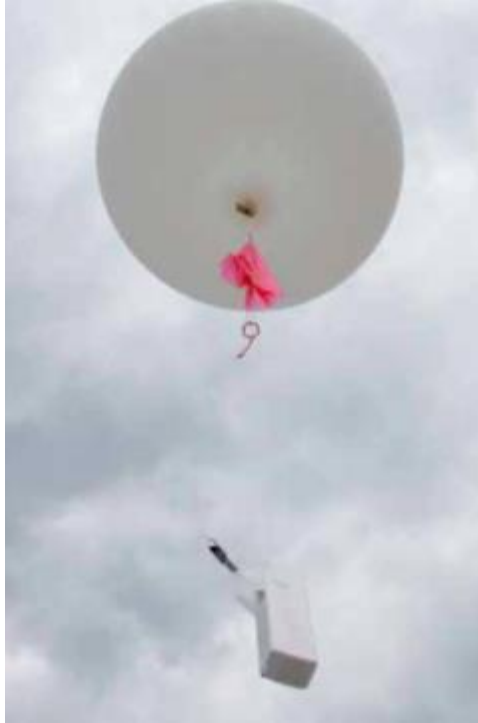
Figure 2: Radiosonde on a weather balloon (Image Source: GRAW Radiosondes )
