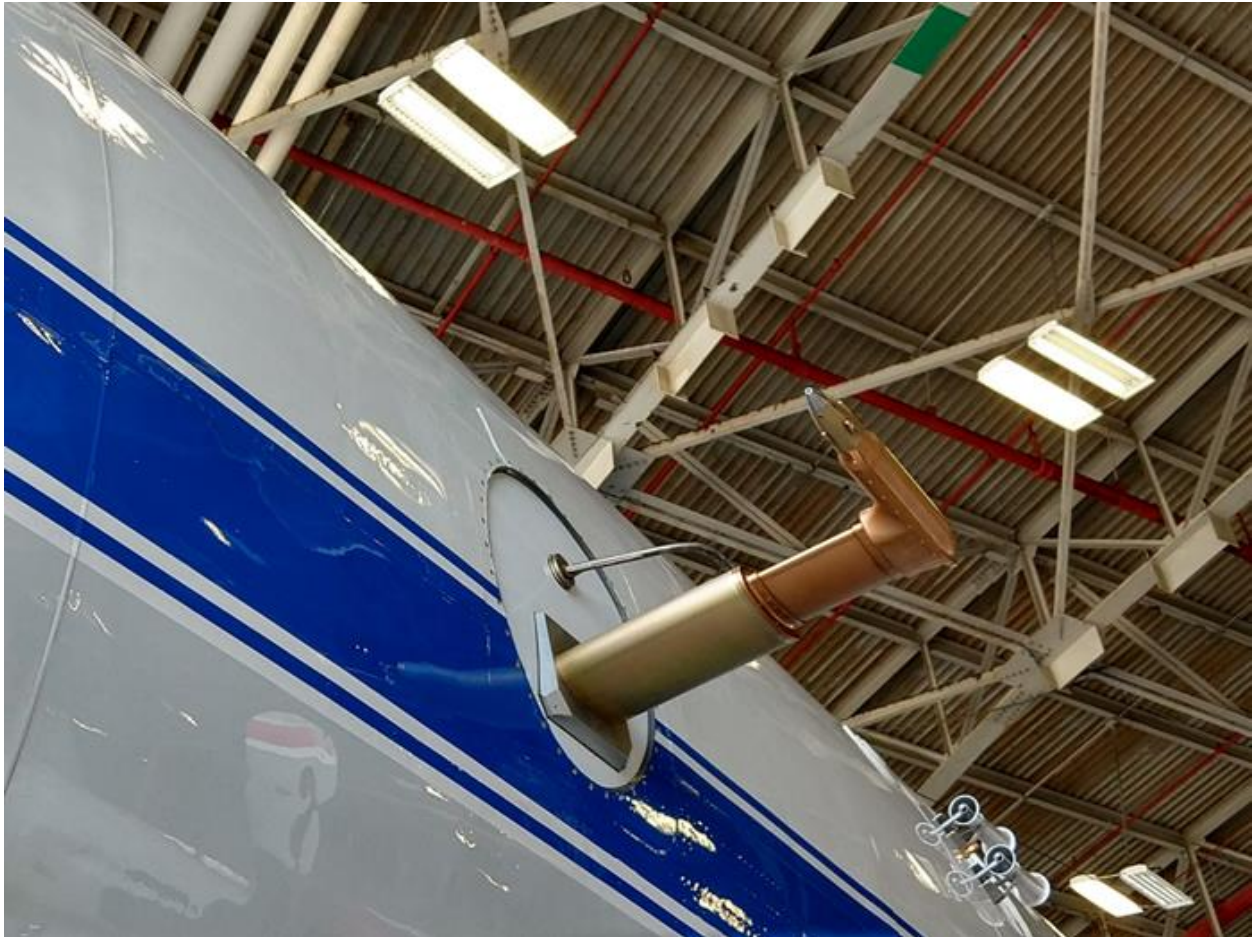
Figure 2: Photo of CVI inlet as deployed on the NASA P-3 for IMPACTS 2020. The front of the NASA P-3 aircraft is to the left in the photo. The CVI inlet faces forward, above which is a backward-facing tube that was used for attempting to measure water vapor in and out of clouds. See text for additional details of both inlets.
