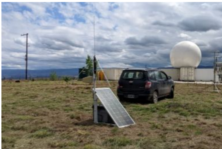
Figure 2: A RELAMPAGO LMA VHF antenna station and associated solar panel. (Image source: RELAMPAGO LMA Data Presentation )
