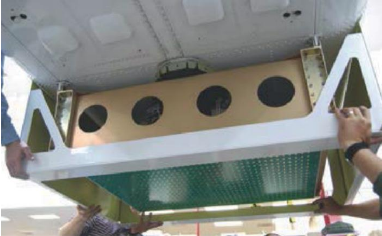
Figure 1: HIRAD system being mounted on the bottom of the WB-57 aircraft (Image Source: Doyle et al., 2017 )
